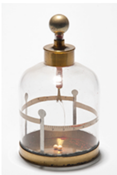
Fig. 3.7 Schlagintweits' 'pith ball electroSCOPE'; source and copyright: History of Science Department, University of Harvard, DW0781; Function: 'This electroSCOPE measures the amount of electric charge on an object. One would touch the object with the brass ball, which would communicate part of the charge to the pith balls inside. The pith balls would then repel each other in proportion to the charge, and this could be quantified by the scales on the wall of the jar. As this particular electroSCOPE is from the Schlagintweit Expedition, it was most likely used for meteorological purposes.' 442
