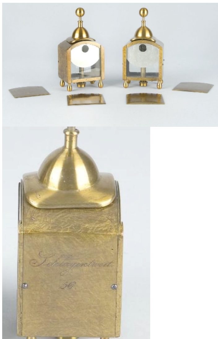
Figs. 3.2-3.3 Schlagintweit, ‘gold leaf electroscope pair’, Material: brass, glass, gold, leather, metal, sheet metal, wood, dimensions: 11.5 x 5.5 x 4.2 cm; source and copyright: History of Science Department, University of Harvard, Inventory Number, DW0780.
