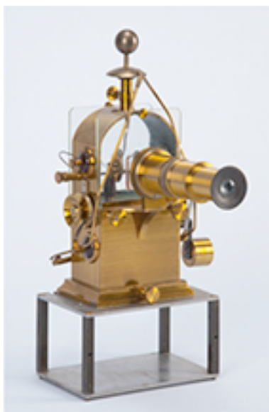
Fig. 3.6. Schlagintweits' electroSCOPE; source and copyright: History of Science Department, University of Harvard, DW0779a. This instrument is used for detecting and measuring electricity. 441
