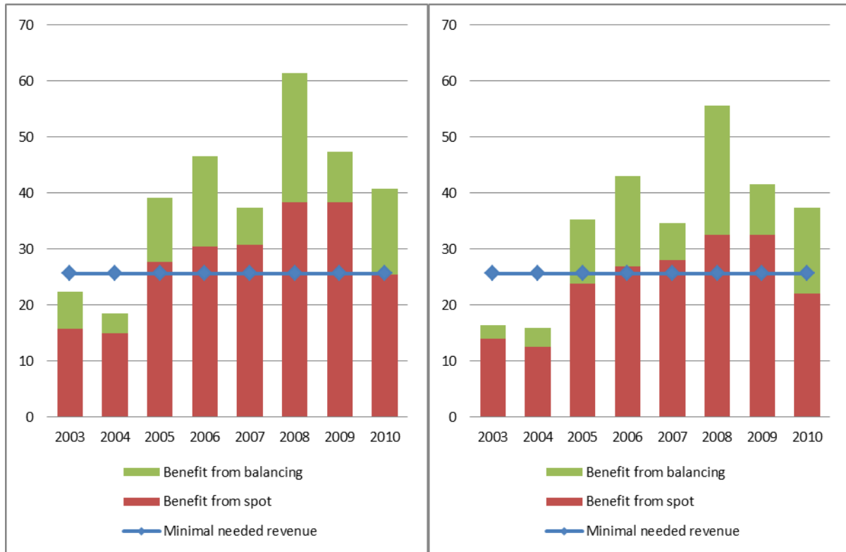
Figures 3 and 4 - Comparison between the minimum annualised investment cost of a demand response program and its annual revenue from the arbitrage between the day-ahead and real time markets between 2003 and 2010 with a 0 % CLPU effect / a 50% CLPU effect
