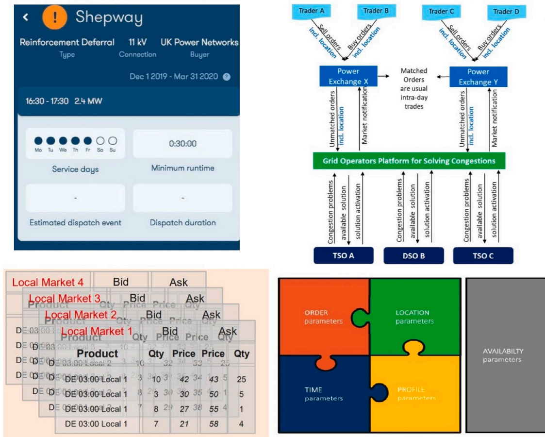
Fig. 1. Illustration of the different short-term market products in Piclo Flex (service window) –upper left, Enera (locational orders) –lower left, GOPACS (IDCONS product) – upper right, and NODES (different types of parameters) –lower right. Sources: Piclo (2019b), USEF (2018), Hirth and Glismann (2018) and NODES (2018).
